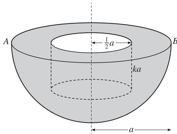
An object is formed by removing a solid cylinder, of height  $ka$  and radius  $\frac{1}{2}a$ , from a uniform solid hemisphere of radius  $a$ . The axes of symmetry of the hemisphere and the cylinder coincide and one circular face of the cylinder coincides with the plane face of the hemisphere.  $AB$  is a diameter of the circular face of the hemisphere (see diagram).
