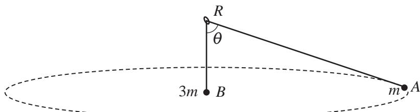
Particles  $A$  and  $B$ , of masses  $m$  and  $3m$  respectively, are connected by a light inextensible string of length  $a$  that passes through a fixed smooth ring  $R$ . Particle  $B$  hangs in equilibrium vertically below the ring. Particle  $A$  moves in horizontal circles with speed  $v$ . Particles  $A$  and  $B$  are at the same horizontal level. The angle between  $AR$  and  $BR$  is  $\theta$  (see diagram).
