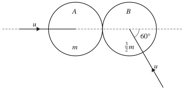
Two uniform smooth spheres  $A$  and  $B$  of equal radii have masses  $m$  and  $\frac{3}{2}m$  respectively. The two spheres are each moving with speed  $u$  on a horizontal surface when they collide. Immediately before the collision  $A$ 's direction of motion is along the line of centres, and  $B$ 's direction of motion makes an angle of  $60^\circ$  with the line of centres (see diagram). The coefficient of restitution between the spheres is  $\frac{2}{3}$ .
